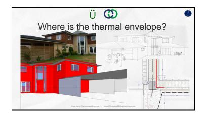
Often at the edge of the slab the insulation pokes in or out a bit. The thermal envelope in PHPP doesn't jog in and out like that. The thermal envelope runs straight vertically down from the outside edge of the wall insulation layer down to the underside of the floor insulation layer. If you confuse this your areas and maybe your thermal bridge calculations need to be redone. It's really important. It's easy to get wrong.
